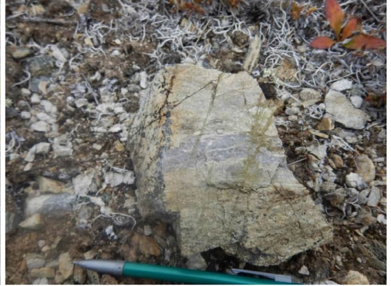
Thin epidote-chlorite veins overprinting quartz-sericite veins within a strongly altered, quartz-sericite-pyrite porphyry from the Maloney area.
