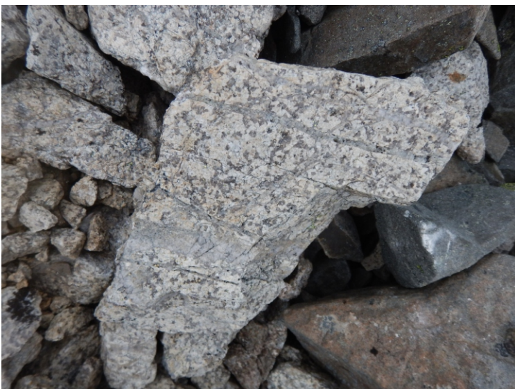
Figure 4. A-type porphyry quartz veins from the Main Ridge zone of the Meloy property. Granodioritic rock is intensely clay altered.
