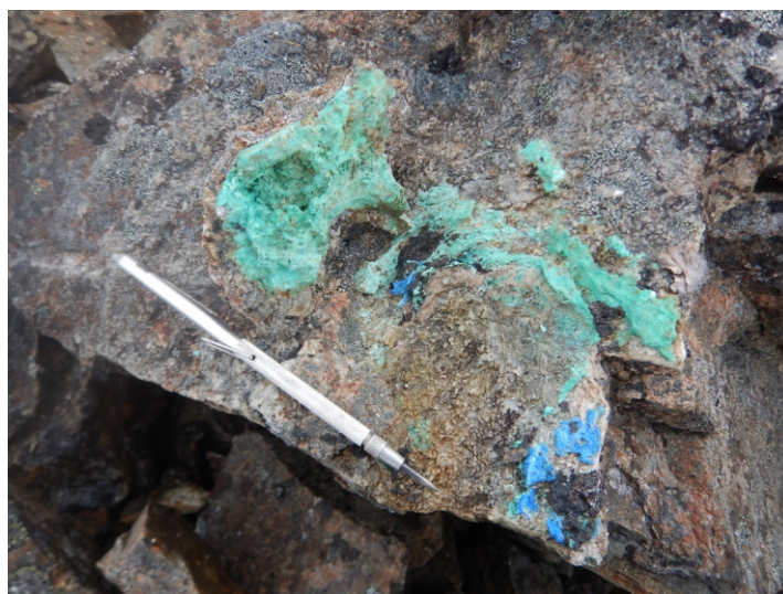
Figure 9. Patchy malachite and azurite after chalcopyrite found at the edges of quartz vein within medium-grained granodiorite.
