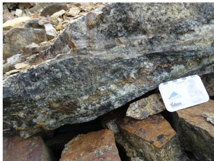
Figure 7. Quartz, chalcopyrite with minor bornite vein within strongly altered granodiorite from the Main Ridge zone.
