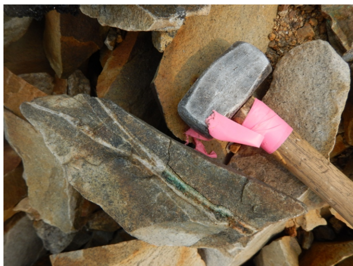
Figure 8. Quartz, chalcopyrite and bornite vein developed within fine-grained, slightly biotite and feldspar porphyritic monzonite.
