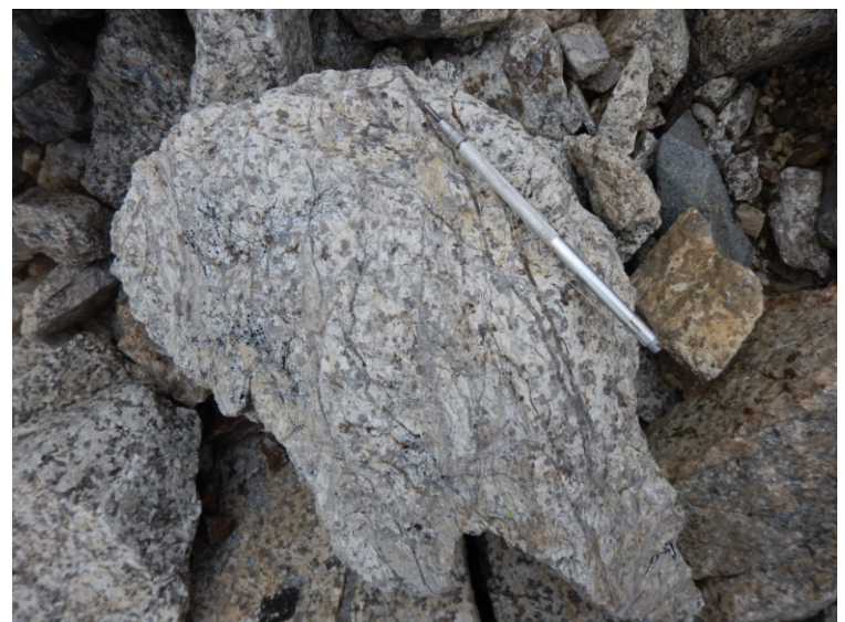
Figure 5. Quartz A-veins and magnetite-quartz veins within granodiorite from the Meloy property. Minor sulphides present in some of the quartz veins.
